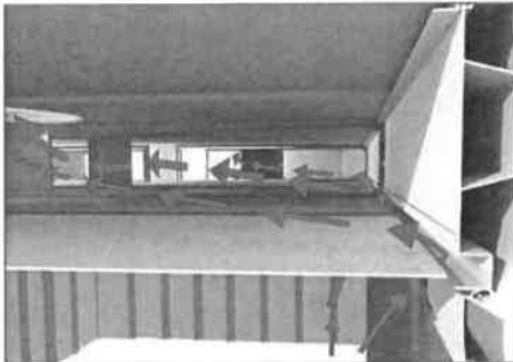
Innovative double panel roof design acts as a baffle, deflector plate and spark arrestor.
