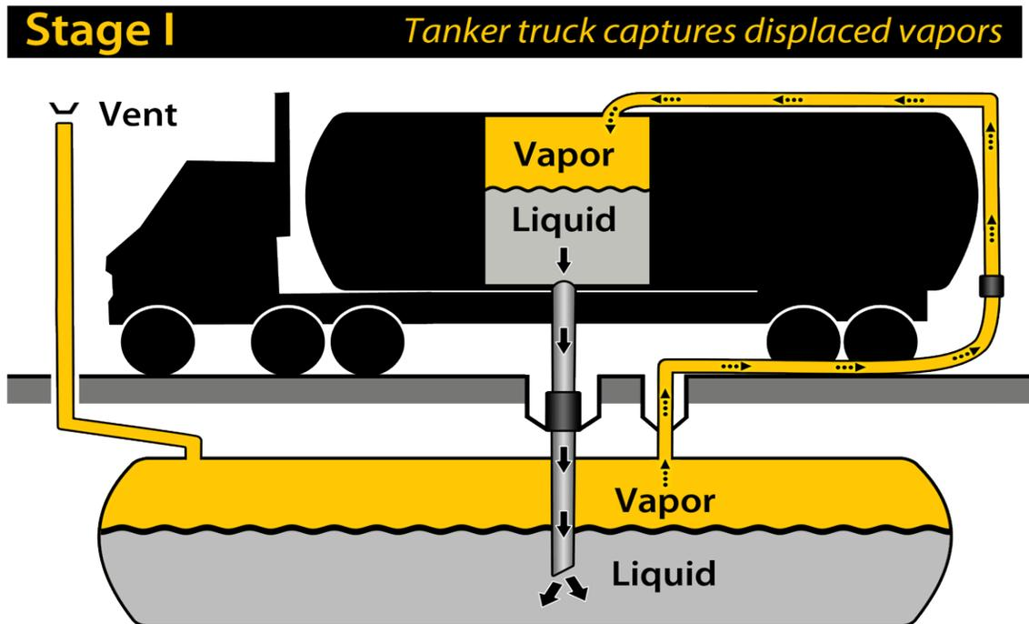
\*Note: Some storage tanks may have one opening that transfers liquid gasoline to the tank and also returns vapor to the tanker.
