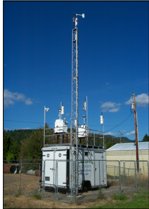
LRAPA monitoring site: one of three sites equipped to collect and log both pollution and meteorological data.
