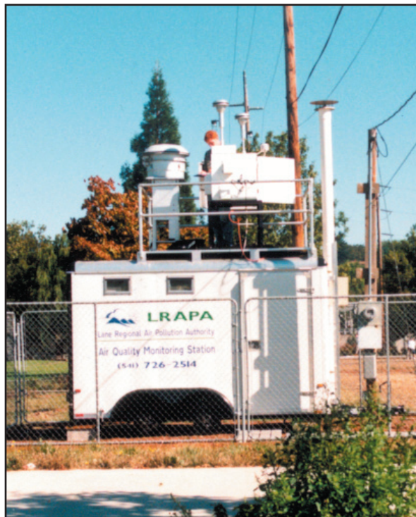
LRAPA monitoring site: one of four sites equipped to collect and log both pollution and meteorological data.
