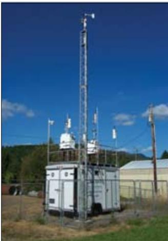
LRAPA monitoring site: one of four sites equipped to collect and log both pollution and meteorological data.
