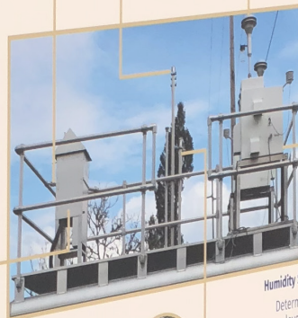
CO and Air Toxic Probe Gauges carbon monoxide and air toxics levels
